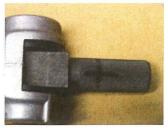
You will need to either press or drive the pin out of the coupler. Using a deep socket, a suitable drift and a hammer, place the coupler on the socket end and drive the pin out using the drift. Once pin is removed, remove the old bushings. Be careful driving out the pin, as the housing may crack if too much force is used.
