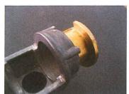
Once you verify the bushing fit, remove them and place them in their correct orientation, inside-out. Use a light lubricant on the outside of the bushings and in the coupler housing to ease installation. Start by fitting the bushings by hand inside the coupler housing and finish by tapping them in using a coin and a suitable drift.
